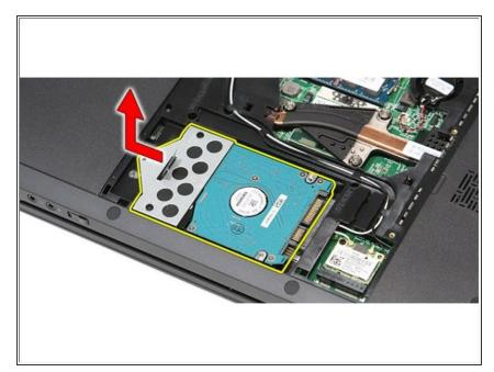
Slide the hard-drive assembly towards the center of the computer and lift it up and away from the computer.
