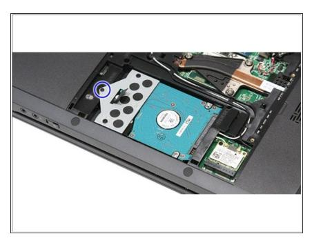
Remove the screw that secures the hard-drive assembly to the computer.
