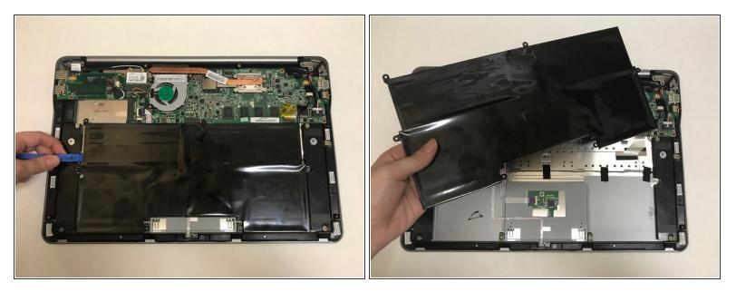
• Use the plastic opening tool or your fingers to pry the battery up and pull it from the laptop.
