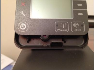
• Removal of the LCD unit: Remove the frame of the LCD unit. You can see the clips for the LCD unit below the push button array. Disengage these to remove the complete LCD unit. pull out the Ribbon cable from the rear of the LCD panel.
