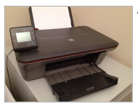
Problem: Screen is blank after start up splash screen. This seems to be a common fault with this printer and in my case was a relatively simple fix. You will need a T10 torx driver and some brute force. Basically there is a push fit ribbon cable that works itself loose on the main PCB. This has to be reinserted for the printer to work correctly.
