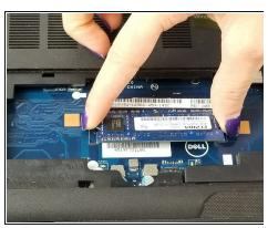
• Remove the memory card by pulling apart the latches holding it in place.
