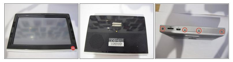
• Using a PH 0 screwdriver, loosen the four screws on the underside of the device.
