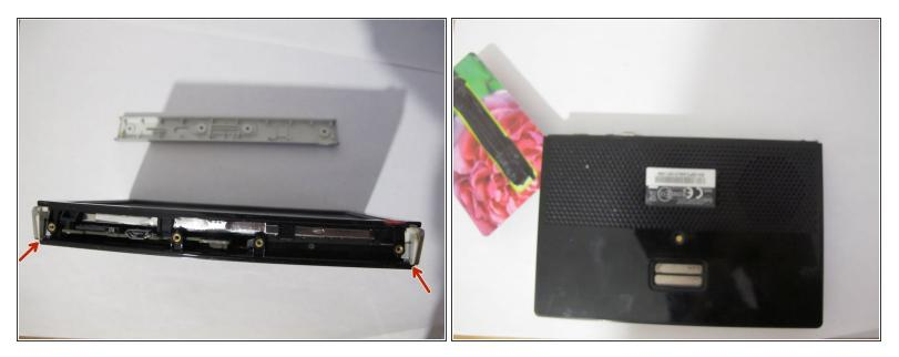
Pull a plastic card between the wall and the side panel to separate them. After the sides also separate the upper edge.
