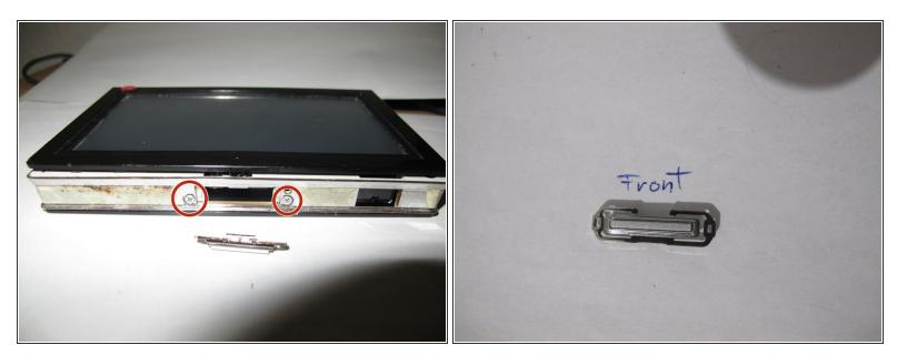
• Use the screwdriver PH 0 to remove the two screws at the upper edge.
