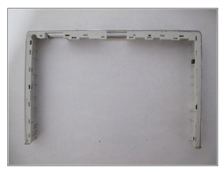
• Pull out the inner edge cover between the screen and the rear panel.
