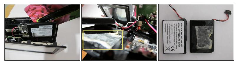
The battery is glued to the housing with a very tough adhesive tape. "Carefully" pry out. (You can probably solve this with isopropyl alcohol - I read later).
