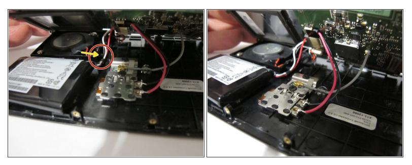
• Pull the battery cable downwards, then out from the guide nose.
