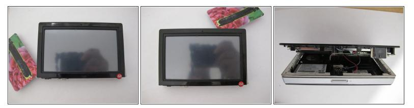
• Pull the plastic card at the lower corners, starting at the bottom of the screen.
