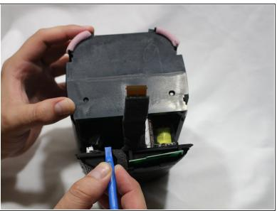
Using a plastic opening tool, separate the motherboard from the speaker.
