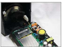
• Using the pointed end of the spudger, disconnect the red, green, and yellow cables connecting the WiFi transmitter/receiver.
