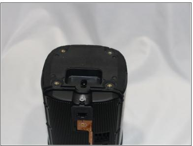
Slide the protective cover upwards to remove.
