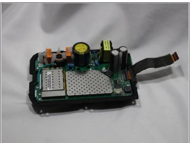
Remove the motherboard panel from the speaker housing.
