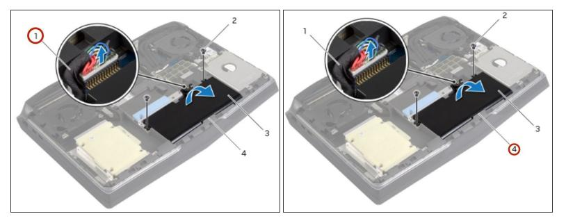
• Using the battery cable, lift and release the battery from the tabs on the computer base.
