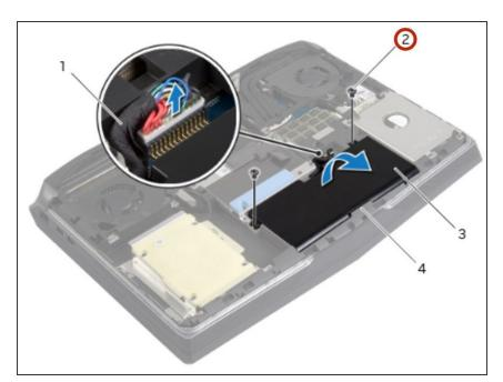
• Remove the screws that secure the battery to the computer base.
