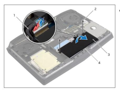
Align the screw holes on the battery with the screw holes on the computer base.
