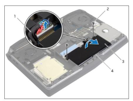
• Replace the screws that secure the battery to the computer base.
