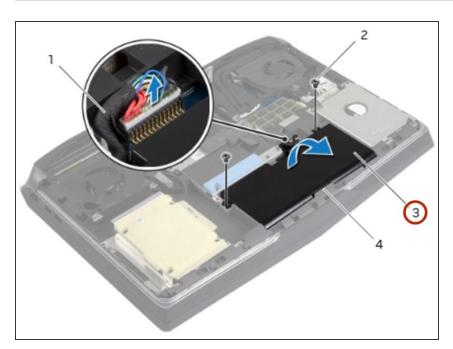
• Slide the **NEW** battery under the tabs on the computer base.
