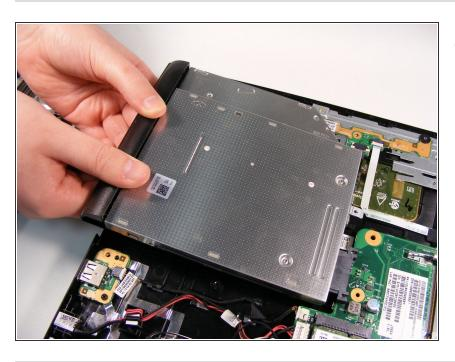
Gently lift up the optical drive at a slight angle, and pull it towards you to remove it.
