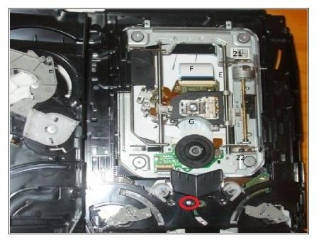
Remove the screw circled in red and lift up the black assembly to reveal the mechanism beneath. Set it aside right-side up and be careful not to shake any parts loose.
