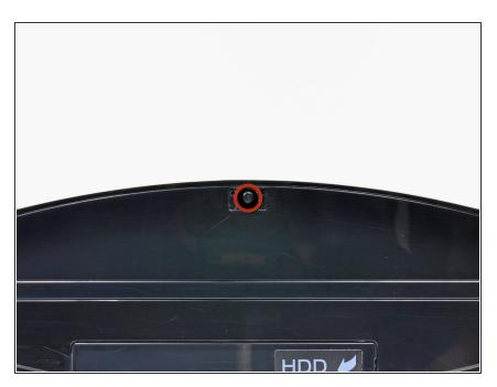
Remove Screw with a TORX Security T10 Bit (or you can use a small flat head screwdriver)
