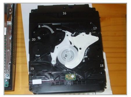
Remove white center hub piece (D) and screws 16 - 20 then fold the top section to the left being careful not to damage the cable to the bottom left. The cable is very delicate and easily damaged.
