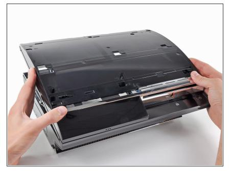
• Lift The Top Casing Towards the front of the PS3 carefully
