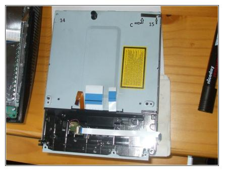
Remove screws 14 and 15 and the silver springboard, slightly bend top metal away from disk entry area, and pull back to remove the metal jacket.
