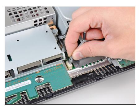
• Carefully Remove Power cable from the motherboard
