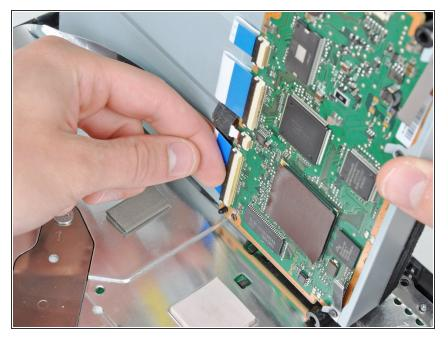
• Lift the Disk drive to the right and remove the largest ribbon cable by lifting the black catch and remove the drive from the PS3
