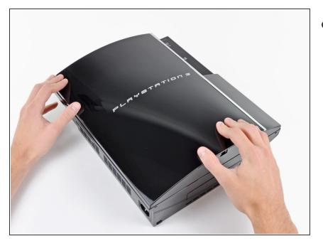
• Carefully slide the top plate and lift to remove
