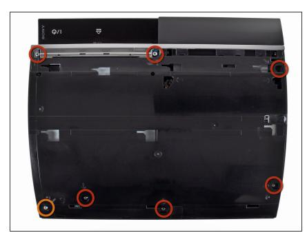
Remove the main screws (philips head)
