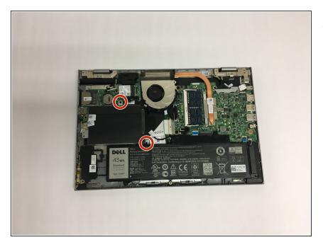
Unscrew and remove the 2 of the 3mm Phillips head screws holding the hard drive in place.
