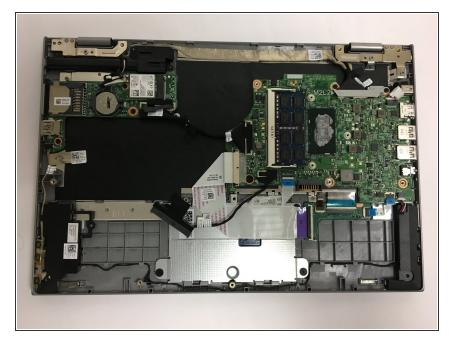
Make sure that the Battery, Hard Drive, and Cooling Fan are safely removed.
