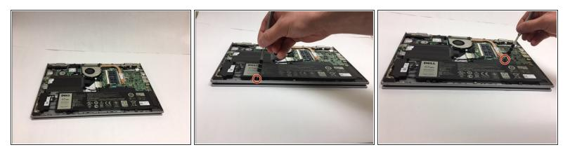
• The battery will be the largest black component in the device located near the bottom edge. Using a Phillips #0 screwdriver, unscrew the two 3mm Phillips head screws holding in the battery.
