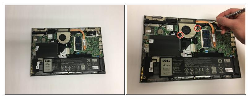
Unscrew and remove the 2 of the 7mm Phillips head screws holding the cooling fan in place.
