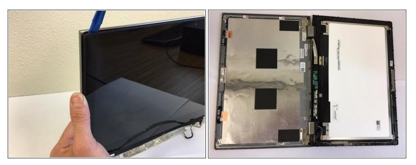
• Using a plastic spudger carefully separate the casing of the screen.
