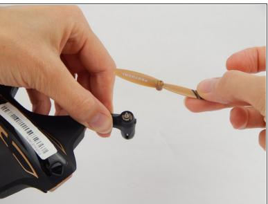
• Use a moderate amount of force to pry the propeller out of its base. The propeller should pop off.
