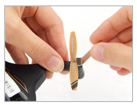
Place a prying tool under the base of the propeller.
