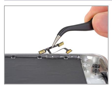
Remove the dual microphone assembly.
