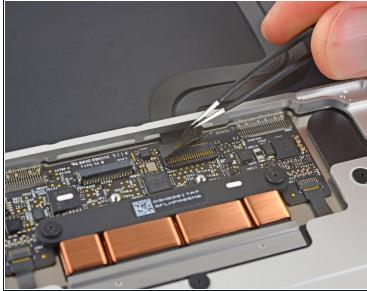
Use a pair of tweezers to remove the tape covering the keyboard ribbon cable connector on the trackpad.
