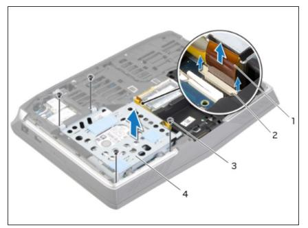
Replace the screws that secure the secondary hard-drive to the secondary hard-drive bracket.
