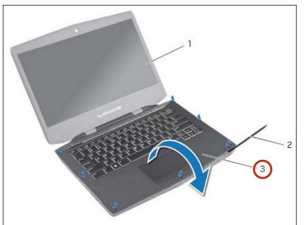
Turn the NEW palm-rest assembly over and slide the status-light board cable through the slot on the computer base.
