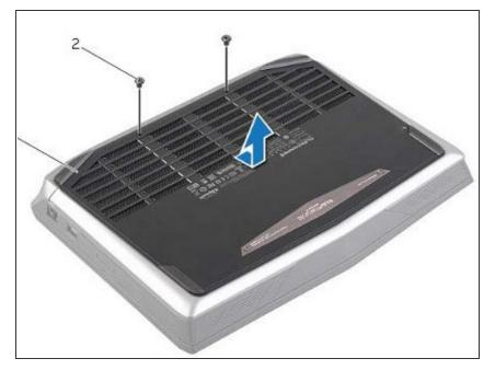
• Replace the screws that secure the base cover to the computer base.
