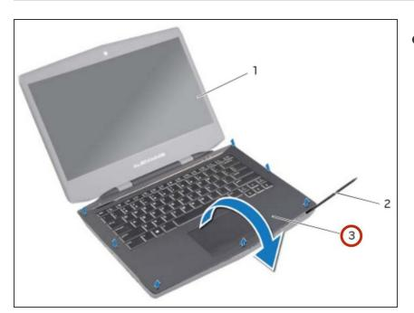
• Carefully lift the palm-rest assembly and turn it over.
