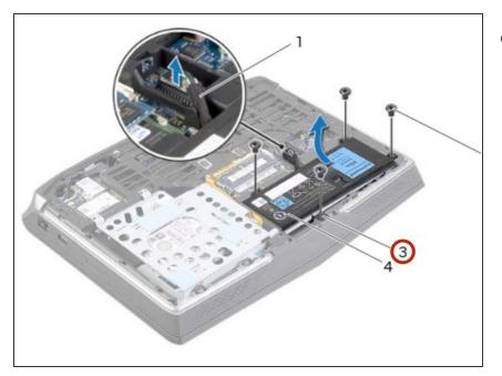
• Align the tabs on the **NEW** battery with the slots on the computer base.
