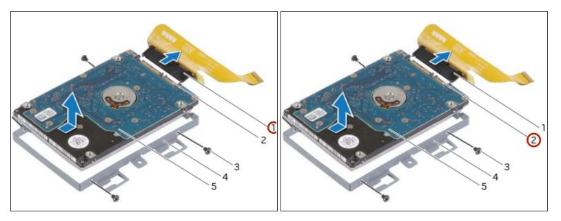
• Disconnect the interposer from the secondary hard-drive connector.
