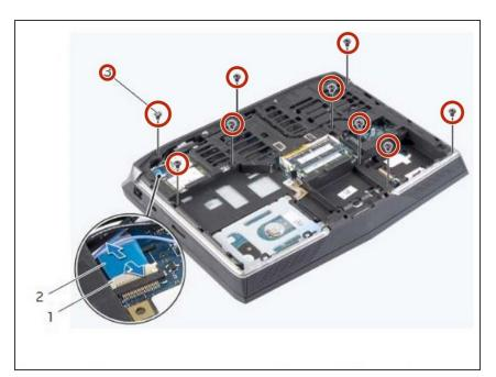
• Replace the screws that secure the palm-rest assembly to the computer base.
