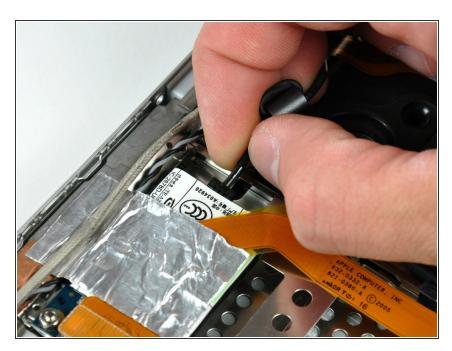
Disconnect the RJ-11 cable from the modem.
