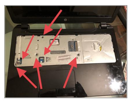
Unhook the 2 connectors and remove the 4 screws.
