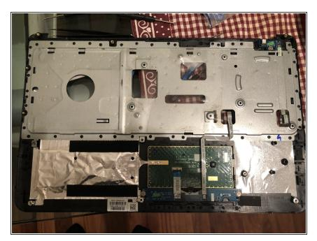
It is possible to remove the upper cover which is free of screws and only hooked by a joint with the help of a thin tool.
