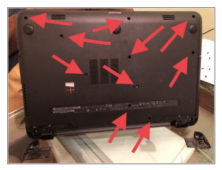
Remove all visible screws at the bottom.
