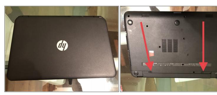
Remove the battery by moving the points marked with an arrow towards the inside.
