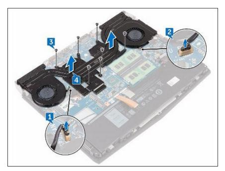
• Disconnect the right-fan cable from the system board.
