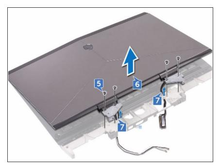
• Lift the display assembly off the palm-rest assembly.
