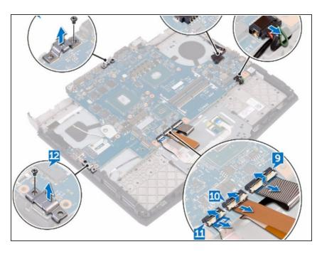
Slide the keyboard-backlight cable into the connector on the system board and close the latch to secure the cable.
