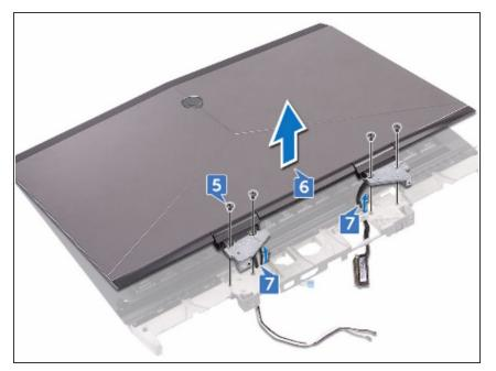
Remove the four screws (M2.5x6L) that secure the display assembly to the palm-rest assembly.
