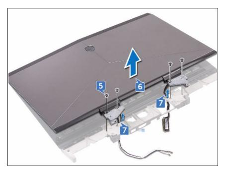
Align the screw holes on the display hinges with the screw holes on the palm- rest assembly.
