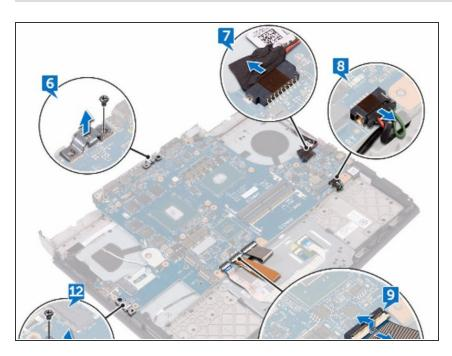
• Open the latch and disconnect the touch-pad cable from the system board.
