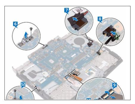
Replace the screw (M2.5x6L) that secures the USB Type-C port bracket to the system board on the back and right side of your computer.
