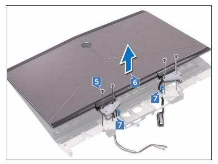
Replace the four screws (M2.5x6L) that secure the display assembly to the palm-rest assembly.
