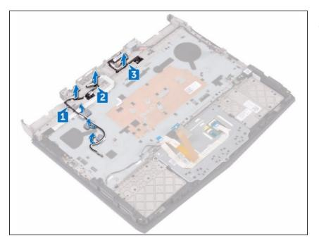
Remove the display cable from the routing guides on the palm-rest assembly.
