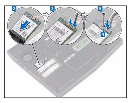
Align the screw hole on the wirelesscard bracket with the screw hole on the wireless card and the computer base.
