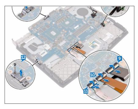
Remove the screw (M2.5x6L) that secures the USB Type-C port bracket to the system board and lift the USB Type-C port bracket off the system board.
