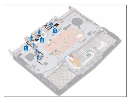
• Remove the logo-board cable from the routing guides on the palm-rest assembly.
