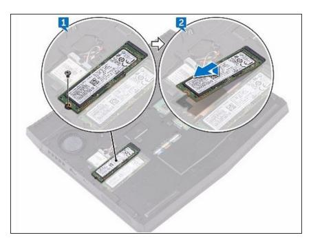
• Lift and slide the solid-state drive from the solid-state drive slot.
