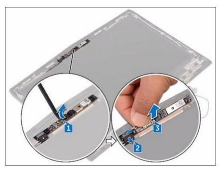
Peel the tape that secures the camera cable to the camera module and disconnect the camera cable from the camera module.
