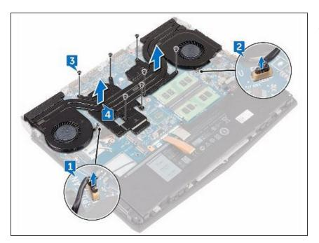
In sequential order (as indicated on the heat-sink assembly), remove the seven screws (M2x3) that secure the heat-sink assembly to the system board.
