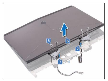
• Remove the cables from the routing holes on the palm-rest assembly.
