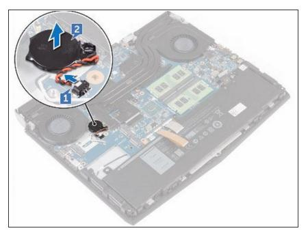
Gently peel off the coin-cell battery along with its cable off the palm-rest assembly.
