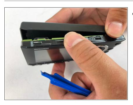
Once unclipped, separate the back casing from the device.
