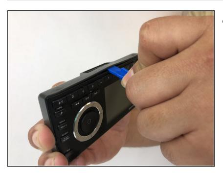
Wedge a plastic opening tool in between the case.
