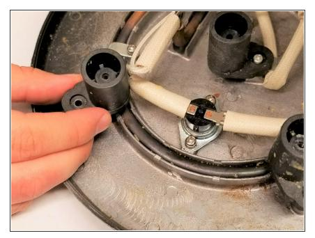
Underneath the heating element are 4 black stands that provide stability by ensuring space between the bottom of the pan and the dipping plate.
