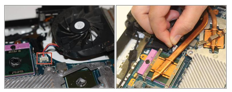
Using your fingers, grasp the white tab and firmly, yet gently, pull up on the wire to disconnect it from the motherboard.
