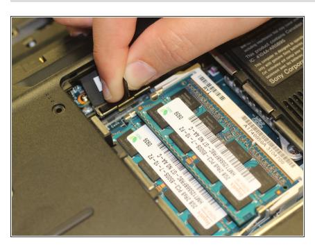
Using your fingers, grasp the black tab and lightly pull up on the ribbon cable to detach it from the motherboard.
