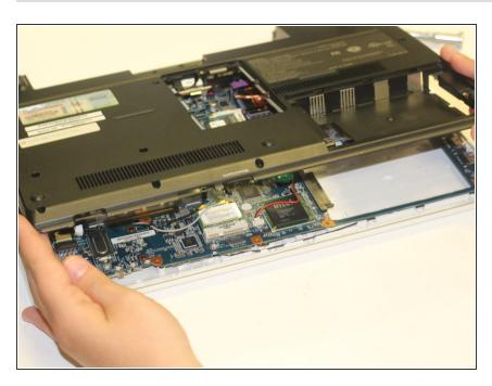
After proper removal of all necessary screws, gently lift up on the back case to remove it.
