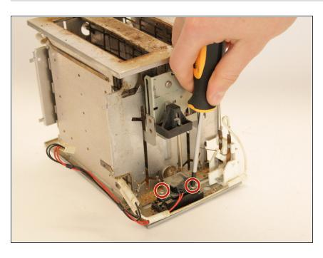
Unscrew the two 10 mm crosshead screws that connect the black wire part to the bottom of the core.
