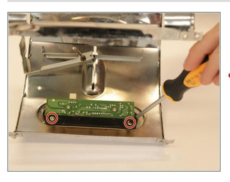
Remove the electric circuit board from the top cover by unscrewing the two 4 mm screws attaching it.
