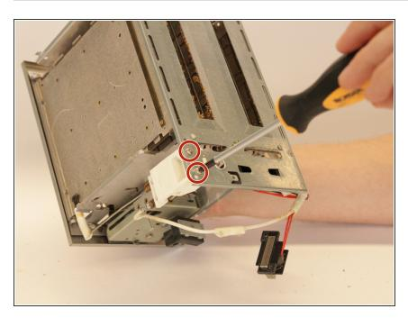
Unscrew the two 10 mm crosshead screws from the white part that is attached to the top of the core.
