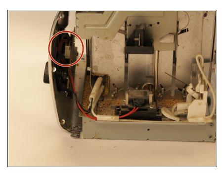
Unplug the ZIF connector from the circuit board.
