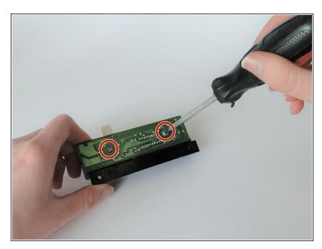
Removed the circuit board from the plastic black part holding it by unscrewing the two 8 mm crosshead screws.
