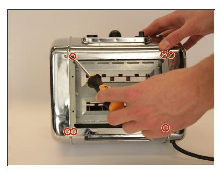
Unscrew the six 5 mm crosshead screws visible on the plate underneath the bottom plate. Use the same crosshead screw driver you used for the bottom plate.
