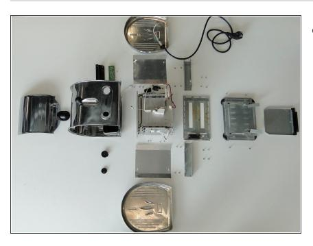
To further dissamble the toaster you will need to twist more metal clips and break the pop nails that hold the base plate and some other parts together. We did not go further since for repair you will probably not need to disassemble the product further. Therefore this is our final exploded view of our disassembly.
