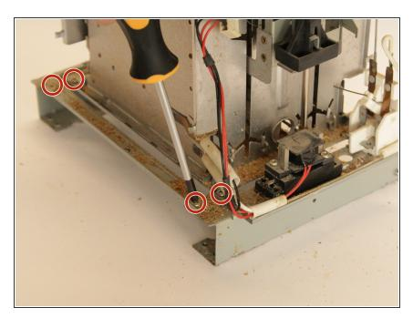
Unscrew the eight 8 mm crosshead screws from the bottom of the core to remove the two legs from the base.
