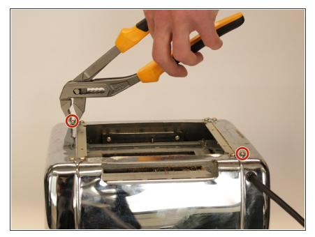
Unscrew the two 5 mm triangular screws with the triangular screwdriver. Again; use a set of pliers or a pipe wrench to get them loose if you cannot get it done with the screwdriver.
