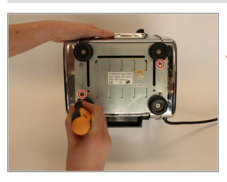
Use a crosshead PZ #1 screwdriver to unscrew the bottom left and top right 5 mm crosshead screws.
