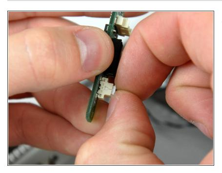
Use your fingernails to pull the microphone connector straight away from its socket on the sound card.
