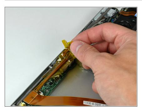
If necessary, remove the strip of tape covering the speaker cable.
