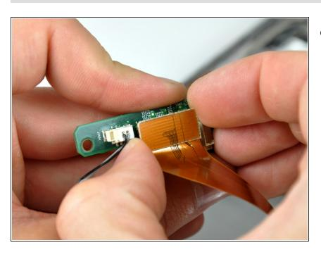
Pull the sound card ribbon cable straight away from its socket on the sound card.
