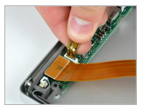
Pull the speaker cable connector straight up to disconnect it from the sound card.
