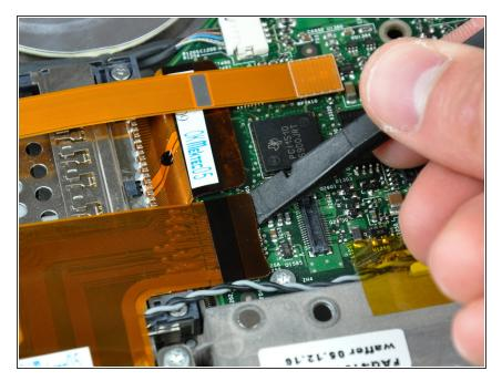
Use the flat end of a spudger to pry the hard drive ribbon cable connector up off the logic board.
