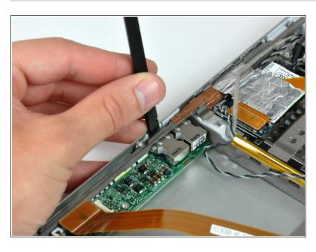
Use the flat end of a spudger to pry the USB sockets away from the left edge of the lower case.
