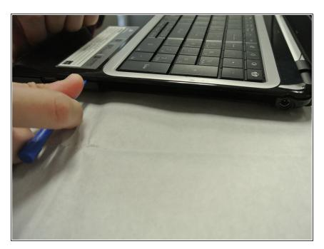
Use a plastic opening tool to pry open the sides of the laptop base starting closest to the hinges.
