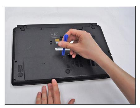
Use a plastic opening tool to pry open the rectangular panel the 9.0 mm screw was removed from.
