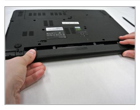
Pull the battery out, making sure to pull the battery parallel to the device.
