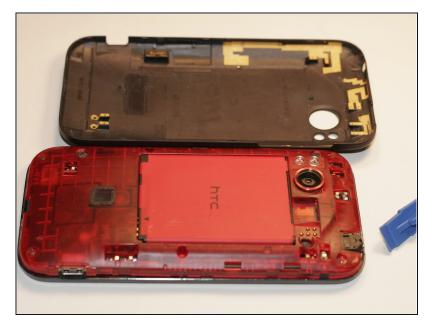
Use a plastic opening tool or your fingers to get into the groove between the cover and case. Remove the back covering so that the red battery is visible.
