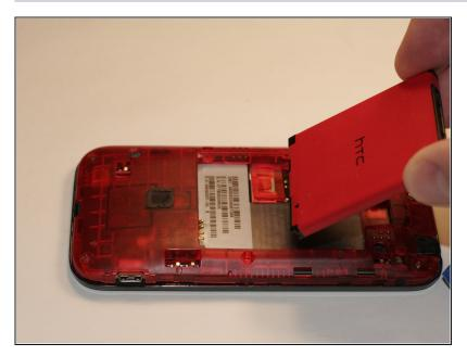
Remove the red battery to replace.
