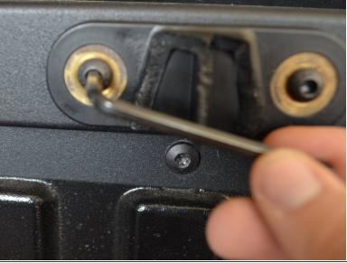
Continue loosening the screws until they are both loose enough to remove by hand.
