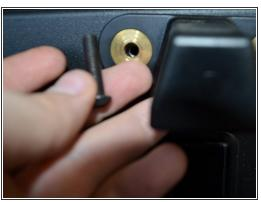
• Hand tighten both of the bolts onto the new latch.
