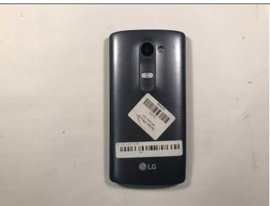
First, make sure to turn the phone over so that you are viewing the backside. The battery is located inside the back of the phone.
