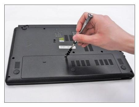
Use a PH0 Phillips head screwdriver to remove the 9.0 mm screw on the rectangular panel underneath the device.
