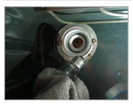
Using a dry cloth or gloves, unscrew the light bulb by turning it in a counter clockwise motion.
