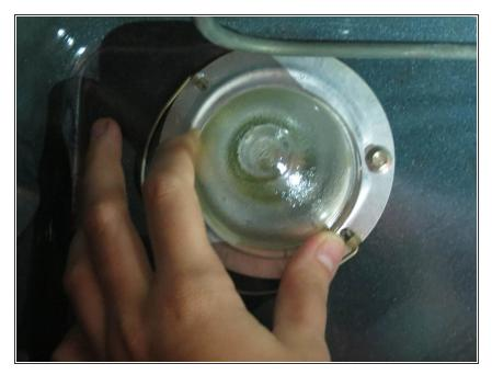
Replace the glass cover over the bulb, but be sure to hold on to it tightly.
