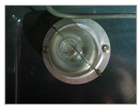
Secure the glass case to the oven with the metal strap by sliding it back over case until it fits tightly.
