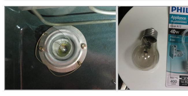
Screw in new light bulb in the clock wise direction.
