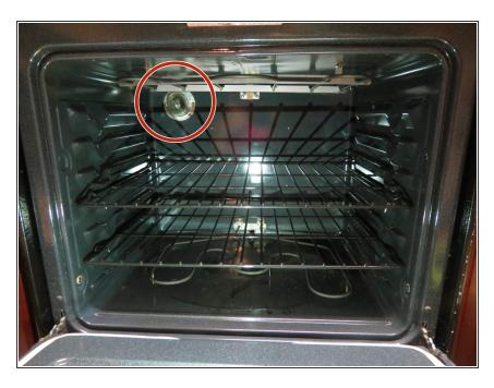
Open the oven door and locate the oven light placement (located on the back wall, in upper left corner for this specific model.)
