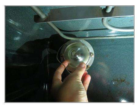
Slide the strap to the side to free the glass casing.
