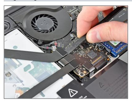
Use the flat end of a spudger to pry the AirPort/Bluetooth ribbon cable connector up from its socket on the logic board.
