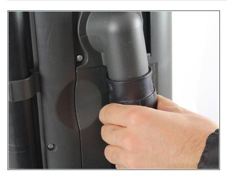
Next, remove the hose from the connector, near the top of the vacuum's rear. This can be achieved by twisting and then pulling down.
