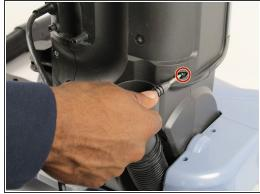
• Use a Phillips #1 screwdriver to remove the 6 screws on the back and bottom of the vacuum shaft.
