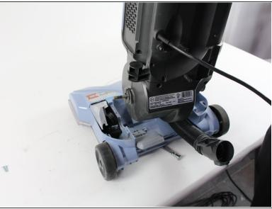
Slide the belt off of the metal rod on the left of the vacuum shaft. Pull the vacuum up and it should easily separate into two pieces.
