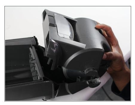
The top of the motor casing should then fold open, revealing the motor.
