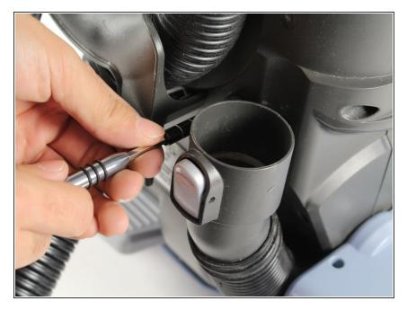
Use a Phillips #1 screwdriver to remove the two screws that secure the hose-release tab.
