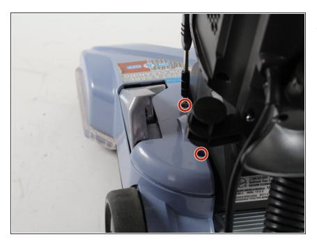
Use a Phillips #1 screwdriver to remove the two screws on the top of the vacuum holding the tab on the left of the vacuum.
