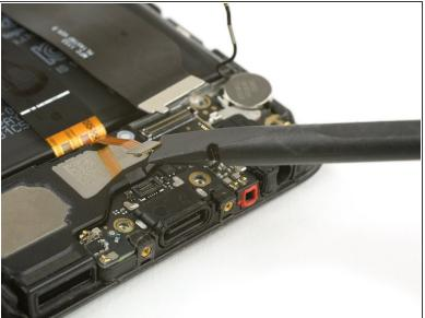
Use a spudger to disconnect the headphone jack and the loudspeaker flex cables.
