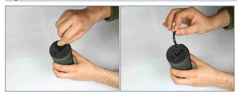
• Remove the rubber port cover, peeling up from one end.
