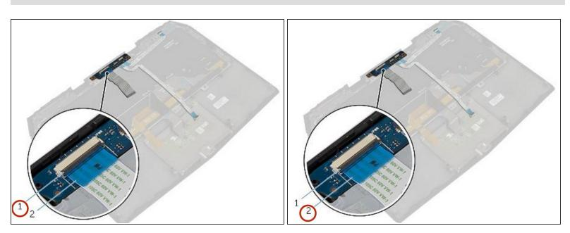
• Lift the connector latch and disconnect the power-button board cable from the power-button board.
