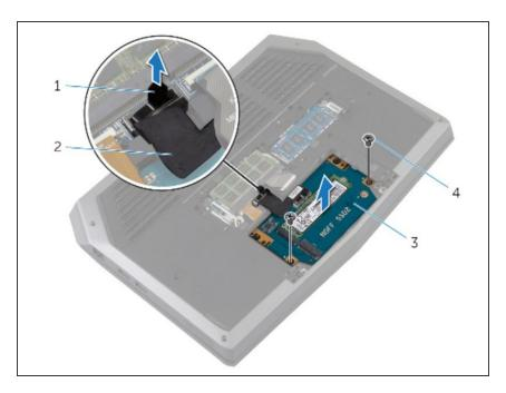
Align the screws on the solid-state drive bracket with the screw holes on the solid-state drive assembly.
