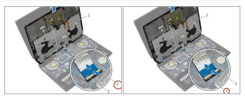
Lift the connector latch and disconnect the power-button board cable from the system board.
