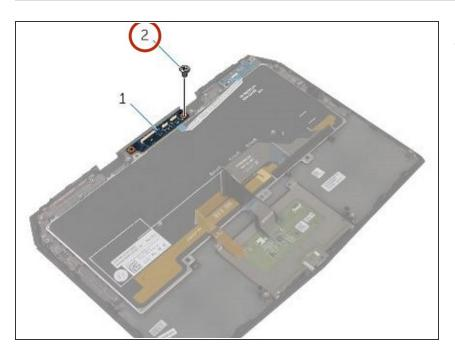
Align the screw hole on the powerbutton board with the screw hole on the palm-rest assembly.
