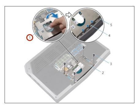
Using the pull tab, disconnect the solid-state drive cable from the system board.
