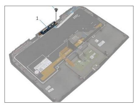
Replace the screw that secures the power-button board to the palm-rest assembly.
