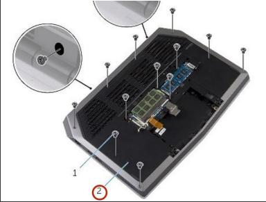
Remove the screws that secure the palm-rest assembly to the computer base.
