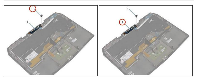
Remove the screw that secures the power-button board to the palm-rest assembly.
