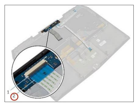
Slide the power-button board cable into the power-button board connector and press down the latch to secure the cable.
