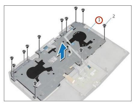
Peel the touchpad cable and statuslight cable off the keyboard bracket.
