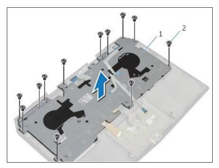
Replace the screws that secure the keyboard to the palm-rest assembly.
