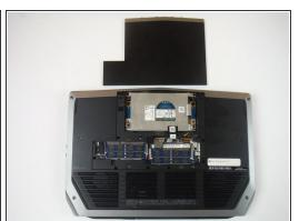
Remove the small access panel using a heavy duty spudger.
