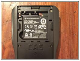
Unscrew the 2 screws on the top of the back of the calculator. Use a Phillips PH00 screwdriver. If your calculator has a lithium ion battery, unplug the cable and gently lift the battery out from the bottom left.
