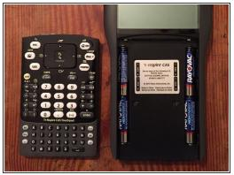
Turn your calculator over and flip the spring loaded switch to the right. The keypad on the front should pop down. Lift the keypad off and take out the 4 AAA batteries.
