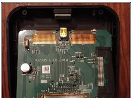
Once you have taken the back plate completely off, unscrew 6 phillips head screws. Remember, these screws are different so keep them separate. After taking the screws out, carefully lift the bottom of the screen up and then the screen and board out.
