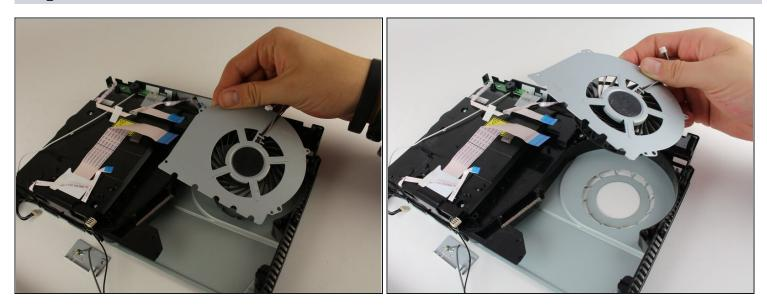
• Remove the fan system by grabbing the edge of the top metal plate and lifting up with your hands.
