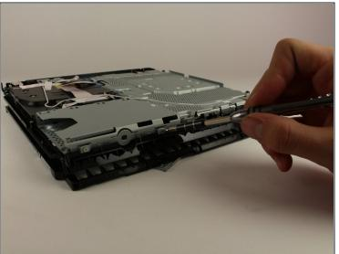
• Unscrew and remove the two 5.0mm screws on the side of the console using a Phillips #1 screwdriver with a counter-clockwise motion.
