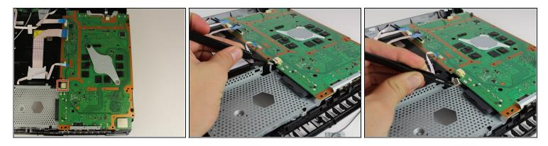
• Remove this wire connection by firmly grasping it with tweezers and pulling out.
