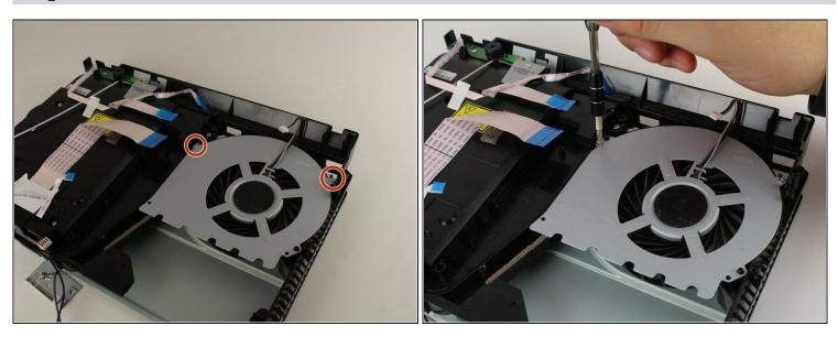
• Unscrew and remove the two 40 mm screws using a PH00 screwdriver with a counterclockwise motion.
