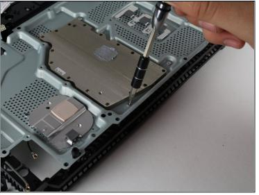
• Unscrew and remove the six 4.0mm screws using a PH00 screwdriver with a counterclockwise motion.
