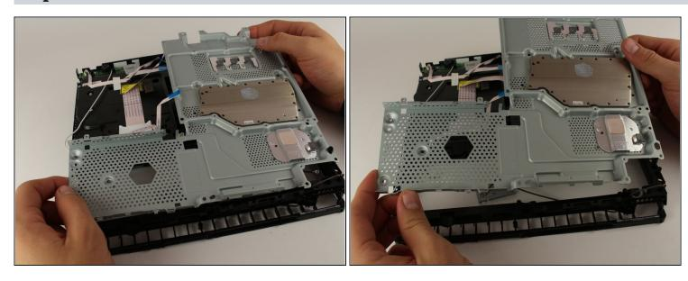
• Remove the metal plate by grabbing the edges and lifting up with your hands.
