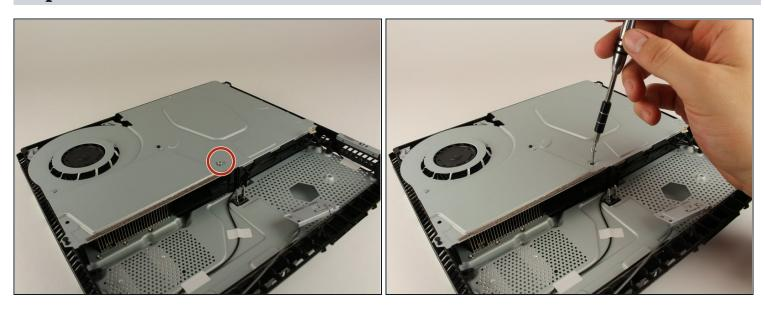
Unscrew and remove the 31.0mm safety screw using a T8 screwdriver with a counterclockwise motion.
