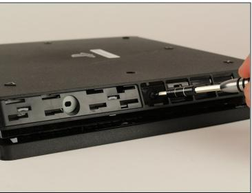
Unscrew and remove the now exposed 5.0mm screw using a T8 security Torx screwdriver with a counter-clockwise motion.
