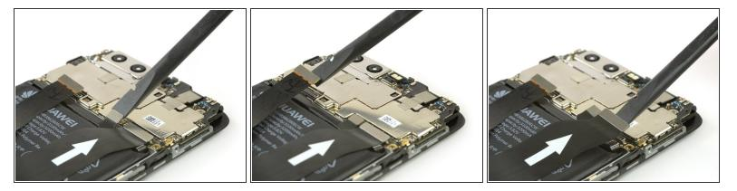
Use a spudger to disconnect the battery, the interconnect and the display flex cable.
