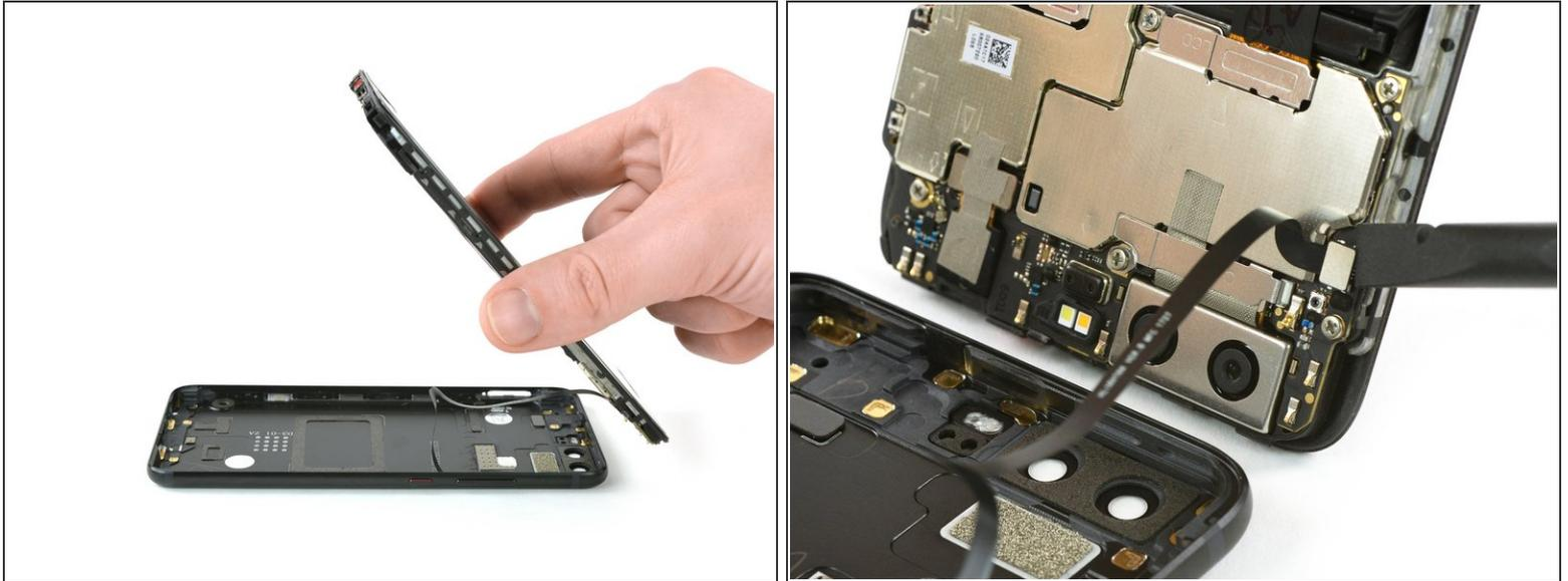
**⚠** Don't open the phone all the way, yet. The cable for the standby and volume buttons is still connected to the back cover.
