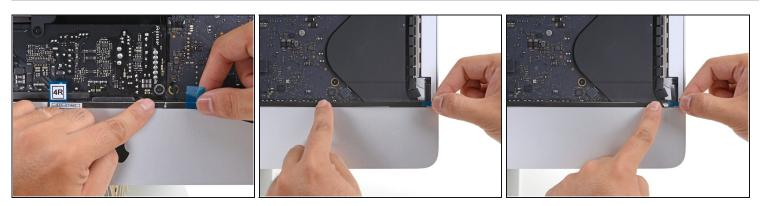
• Run your finger from left to right along the length of the adhesive strip to ensure it is straight and unwrinkled, pressing down as you go to adhere the strip to the iMac.
