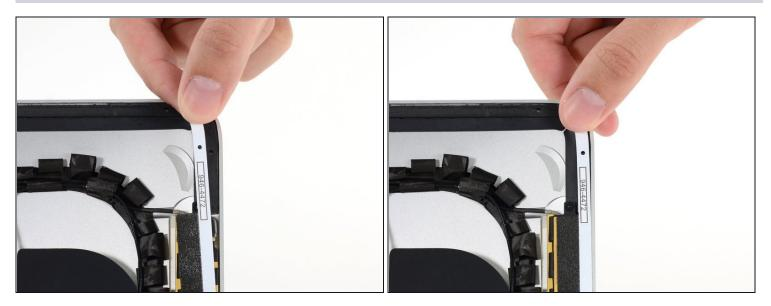
• Align the upper half of the strip with the right edge of the rear enclosure, and stick it down.
