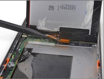
• Use the tip of a spudger to lift the battery connector up out of its socket on the motherboard.
