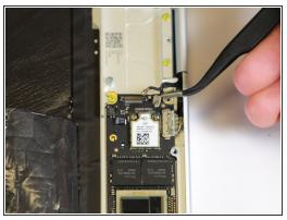
• Disconnect the two black cables from the motherboard by pulling the connectors upward using the needle-nose tweezers.
