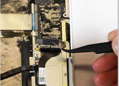
• Using needle-nose tweezers, remove the silver casing by lifting it up and out of the computer.
