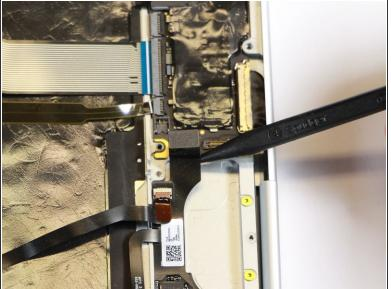
• Disconnect the flat, black cord from the motherboard by using a spudger to push it upwards out of the slot, or by using your hand to carefully pull upward.
