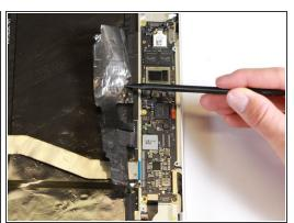
Fold back the plastic covering on the motherboard using the nylon spudger.
