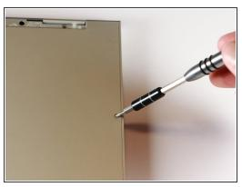
Remove the seventeen 3.0mm T5 Torx screws from the bottom panel.
