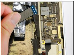
• Disconnect the large flat ribbon cable from the motherboard by using your hand to gently pull it out of the socket, or by using a pair of tweezers to pull it out.
