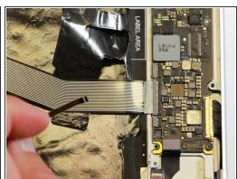
Disconnect the flat ribbon cable from the motherboard by using your hand to gently pull it out of the socket, or by using a pair of tweezers to pull it out.
