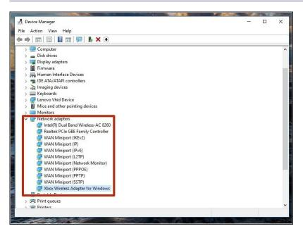
To verify the driver was installed correctly, check under Network Adapters. If the driver was installed correctly, it will show up here.
