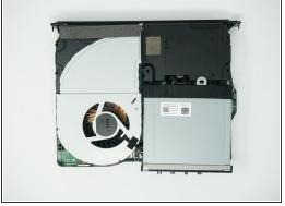
Remove the metal casing by pulling it upward, revealing the interior components of the device.
