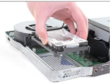
Lift the hard drive assembly up out of the upper metal case.
