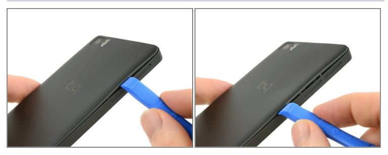
• Insert the tip of an iFixit opening tool between the back cover and the mid frame of the phone.
