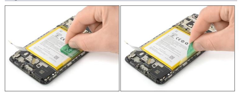
• Peel the green adhesive strip off the battery.
