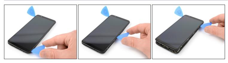
• Slide the opening pick around the bottom right corner and then up along the right edge of the phone to open the plastic clamps that secure the backcover.
