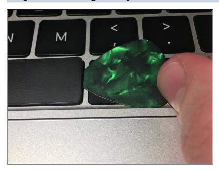
Push the pick **right and down** from its top. This should pull the edge of the keycap up. **Make sure not to push the pick to the left (inwards, under the key) yet**. If you push the pick left too early, it will end up under the scissor clip.
