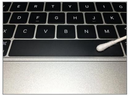
Turn off your MacBook Pro and clean around the space bar using a cotton bud and isopropyl alcohol. This will help to prevent excess dirt from falling under the space bar, which will your problems.
