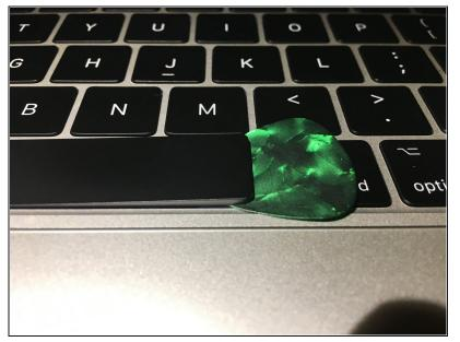
Once the pick is horizontal, push it in towards the centre of the key. You should feel some resistance. Twist the pick and the first clip should pop free. This does not require much force.
