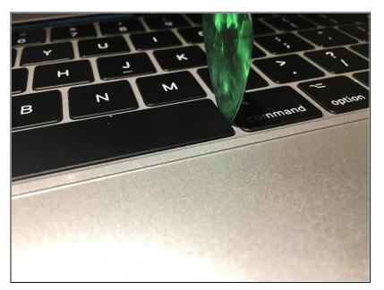
Slide a thin guitar pick or card (not a credit card, most are too thick) vertically down the right edge of the key.
