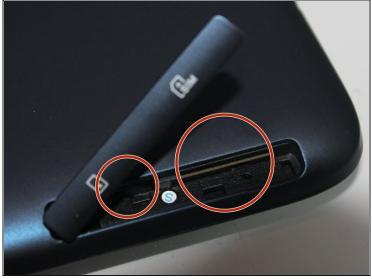
Remove SD and SIM card from device
