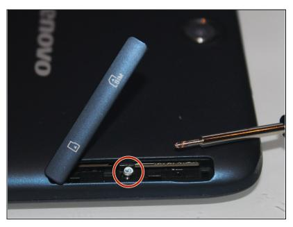
• Remove screw with a simple coss screwdriver
