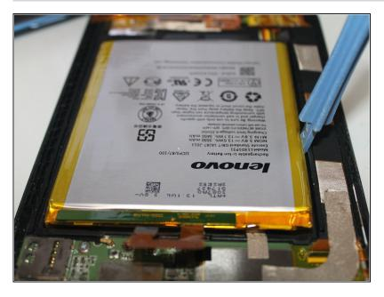
Disassemble battery pack. This might require a bit of pressure as it is glued
