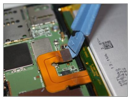
• Remove connection cable as shown.
