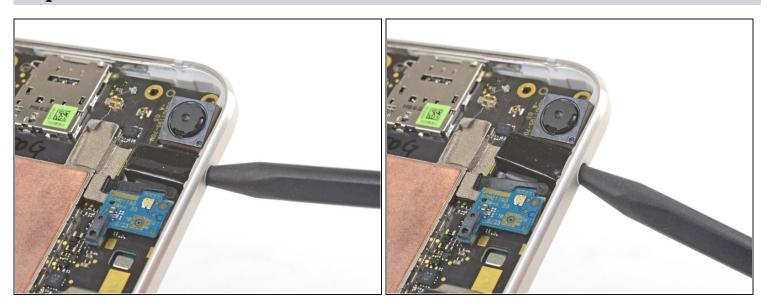
• Insert the point of a spudger into the headphone jack port and pry upwards to loosen the port from its socket.
