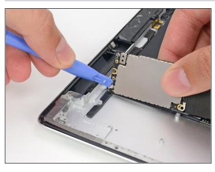
Use a plastic opening tool to disconnect the right antenna cable from its socket on the communications board.
