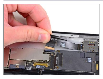
Pull the headphone jack and front camera ribbon cable straight out of its socket on the logic board.
