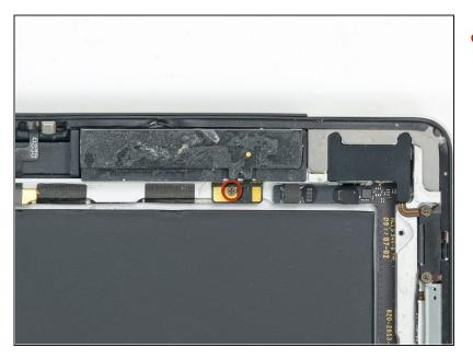
• Remove the single 2.1 mm Phillips screw securing the right cellular antenna to the rear case.
