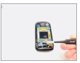
Take a <u>Spudger</u> and push up on the little black bar at the top end of the screen to logic board cable
