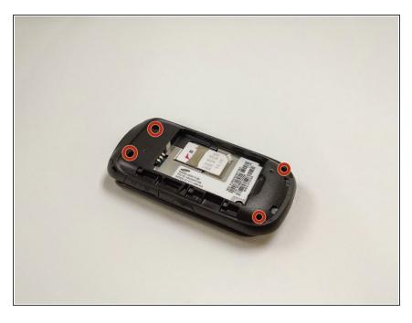
You will see 4 phillips 00 screws, two on the top left and right and two on the bottom left and right. Remove them.
