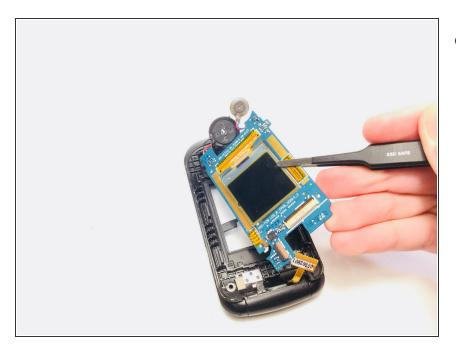
Take a pair of <u>tweezers</u> and lift up to remove the screen.
