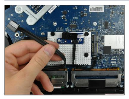
Pull the SATA data cable out of its channel in the logic board and tuck it aside near the left edge of the rear case.
