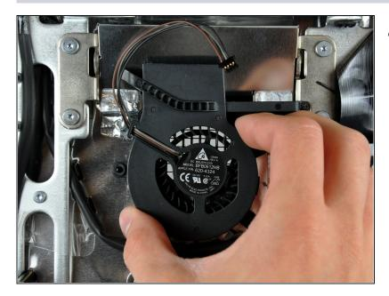
Gently lift the hard drive fan off the plastic posts protruding from the rear case.
