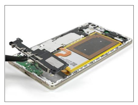
Remove the loudspeaker carefully.
